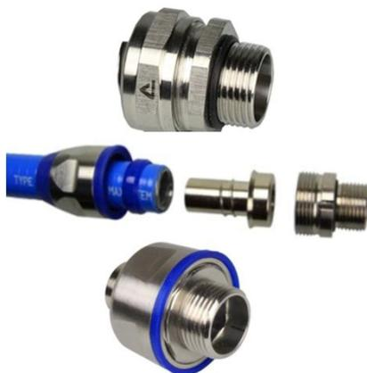
Counter nut, ferrule and body are stainless steel AISI-316. The clamping ring is made of nickel plated brass. O-rings are from NBR. -55 °C till +260 °C.
